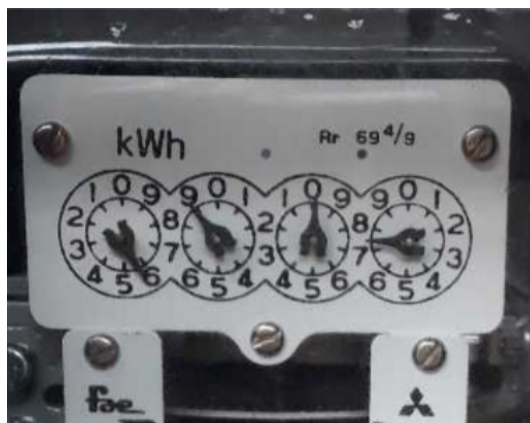
(a) multi-dial meter from UFPR-ADMR
